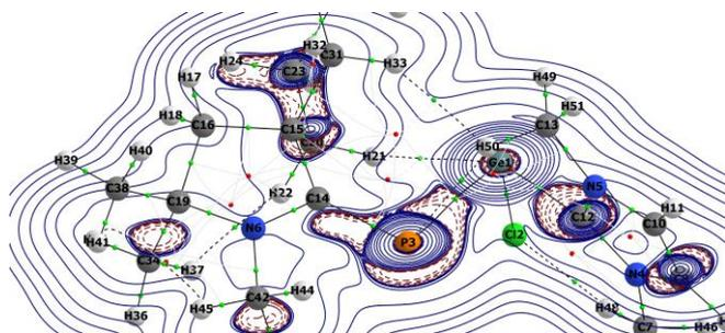
**Figure 5.** Contour plot of Laplacian distribution  $[\nabla^2\rho(r)]$  in the P3-Ge1-C12 plane of **3a'**. Solid blue lines indicate the areas of charge concentration ( $\nabla^2\rho(r) < 0$ ), while dotted purple lines denote charge depletion ( $\nabla^2\rho(r) > 0$ ). Solid lines connecting atomic nuclei (black) are the bond paths.
