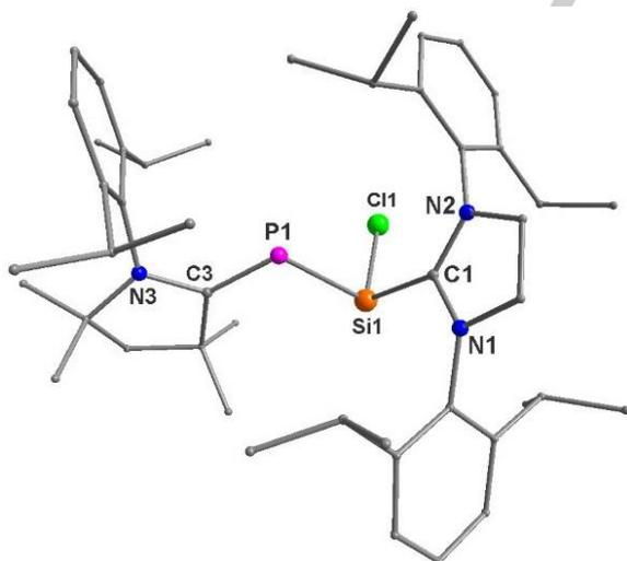
**Figure 3.** Molecular structure of compound (Me<sub>2</sub>-cAAC)P–SiCl(NHC) (**6**). H atoms are omitted for clarity. Selected experimental bond lengths [Å] and bond angles [°]: N3–C3 1.379(6), C3–P1 1.713(5), P1–Si1 2.2951(18), Si1–Cl1 2.1857(17), C1–Si1 1.968(4), C1–N1 1.372(6), C1–N2 1.349(6), N3–C3–P1 122.0(3), C3–P1–Si1 107.32(16), P1–Si1–C1 87.02(14), P1–Si1–Cl1 98.84(7).
