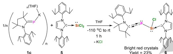
**Scheme 2.** Synthesis of cAAC and NHC-stabilized elusive phosphinidene-chlorosilylene (cAAC)P–SiCl(NHC) (**6**).
